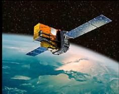
*INTEGRAL*, launched 2002 (ESA), primarily gamma-ray instrument but also wide-field X-ray and optical capability [4 keV - 10 MeV]
